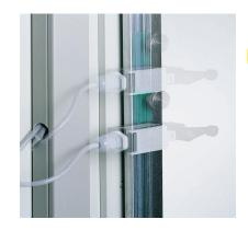
The opening of the press is easily adjusted by the variable limit switch. The limit switch is mechanically adjusted at the guide rail.
